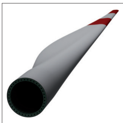
Fig. 3. The outermost layer of the hollow blade fulfills the aerodynamic function
